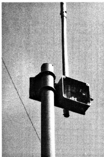
Fig. 4: Photo of PW-50V mounted on a mast. Note: The sleeve joint, visible near the base of the radiating section, is not required and was only used for original development work.
